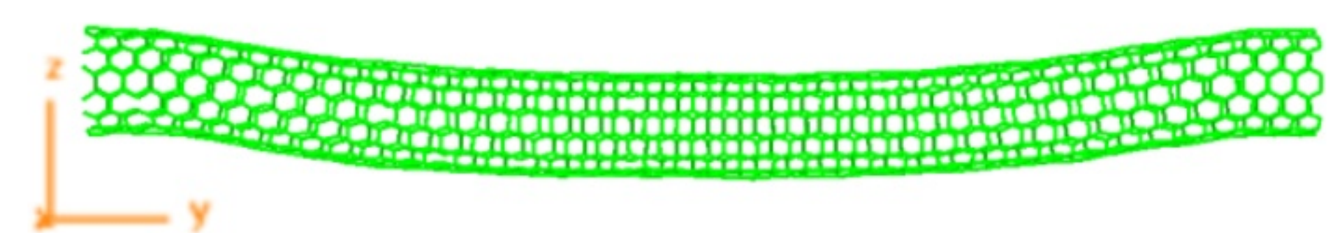
Figure 4: Nanotube vibrating in the Z direction. Three periods at each end are clamped in position.
